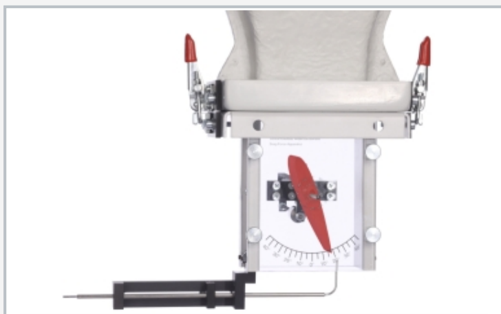
Determining drag in various drag bodies using the accessory HM 225.04
