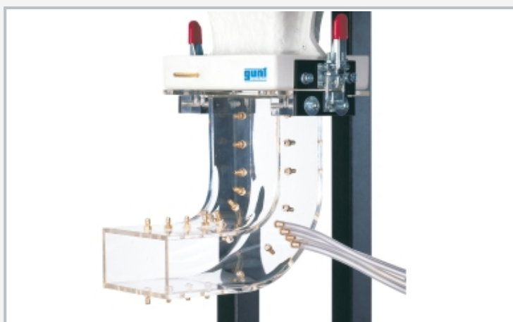
Investigation of flow in a pipe elbow with the accessory HM 225.05
