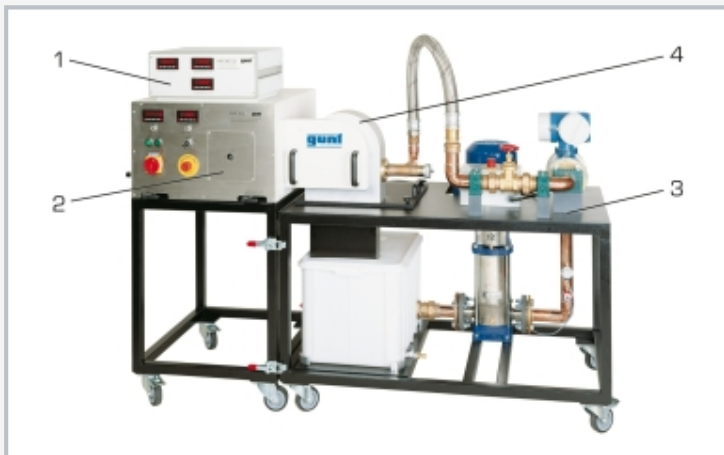
1 measuring amplifier with digital display of measured values, 2 HM 365 Universal Drive and Brake Unit, 3 HM 365.32, 4 HM 365.31 Pelton and Francis Turbine
