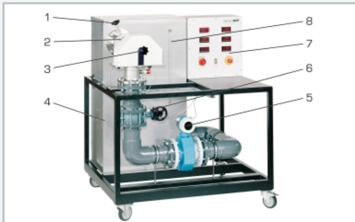
1 lever for adjusting the guide vanes, 2 Propeller type turbine, 3 brake, 4 tank with submersible pump, 5 flow rate sensor, 6 handwheel for throttle valve, 7 switch cabinet, 8 level indicator for tank
