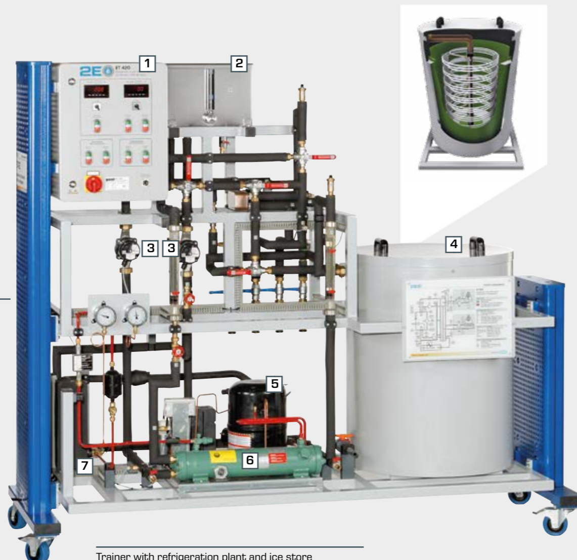
Trainer with refrigeration plant and ice store
