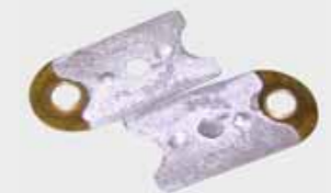
Trip element with melted solder joint
