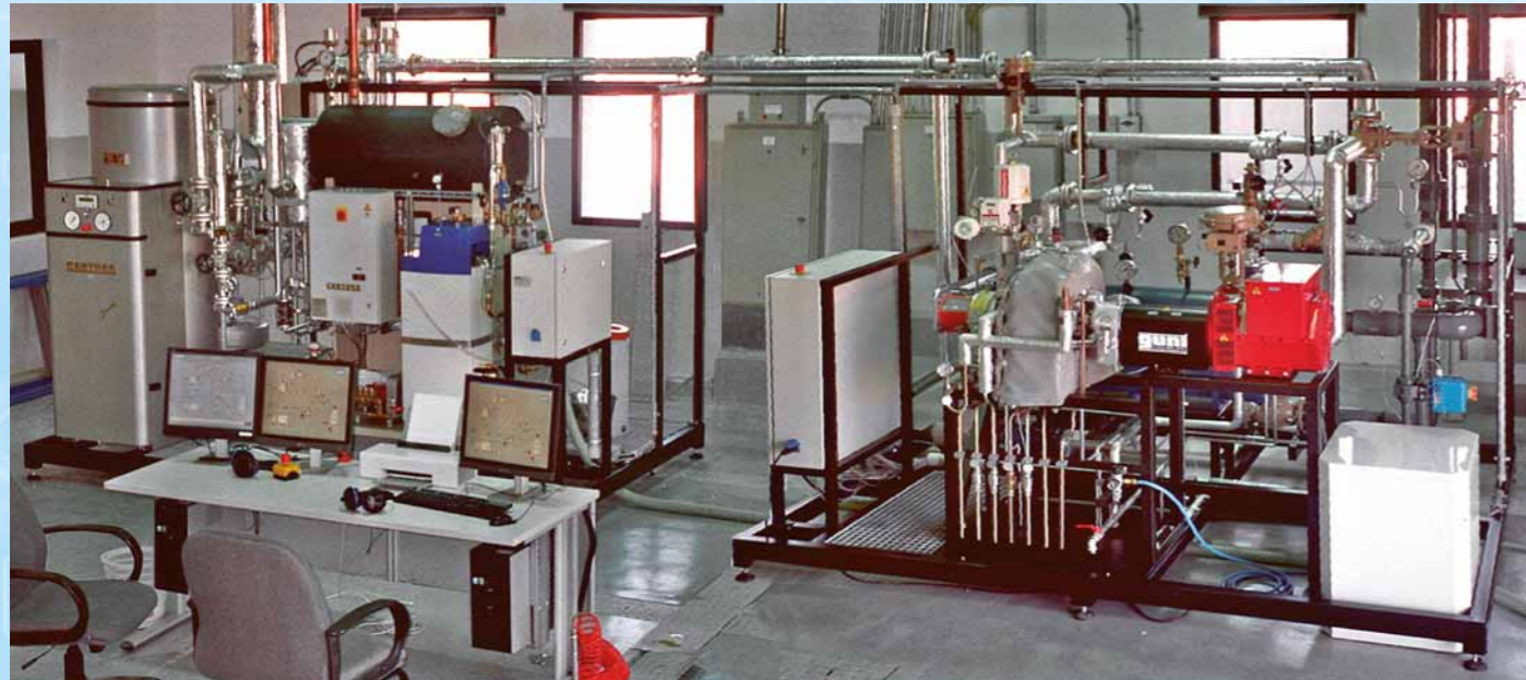
Complete plant consisting of steam generator (left), steam turbine (right) and control station (front)
