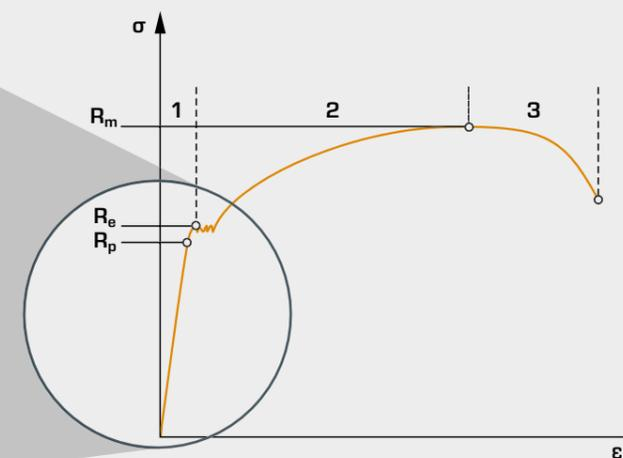
The elastic region is divided into a linear-elastic component a, where the strain is proportional to the stress and is reversible and a nonlinear-elastic component b, where the strain is not proportional to the stress but is still reversible. In the plastic region, the strain is not reversible and the deformation remains even after the force has been removed.
