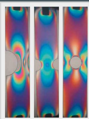
Tensile load with stress concentration on cross-sectional contraction
