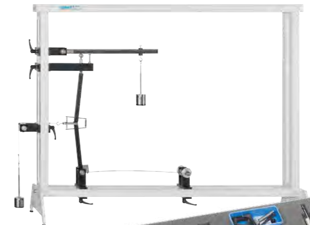
SE 110.19 Investigation of simple stability problems
