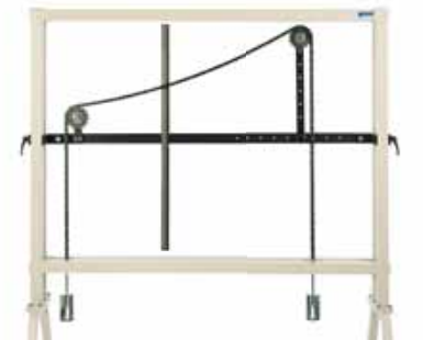
SE 110.50 Cable under dead-weight
