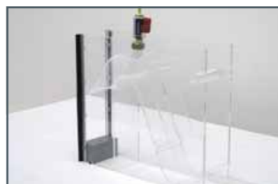
Siphon weir HM 160.36
