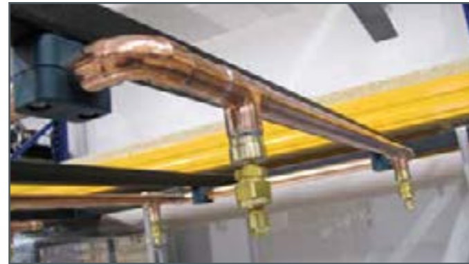
Precipitation device with nozzles for realistic simulation of rainfall
