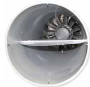
Throttle valve at the end of the measuring section for adjusting the volumetric flow rate
