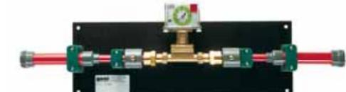
The position is important for correct operation: only horizontal mounting
