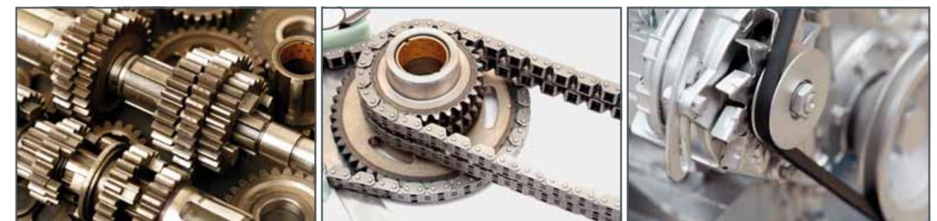
Complex machine elements used to alter the motion variables of path, velocity and acceleration are known as conversion elements or gears. In a gear drive, positively locking **gears** transfer the rotary motion from one shaft to another. In a traction drive, the rotary motion is transferred between two shafts by
