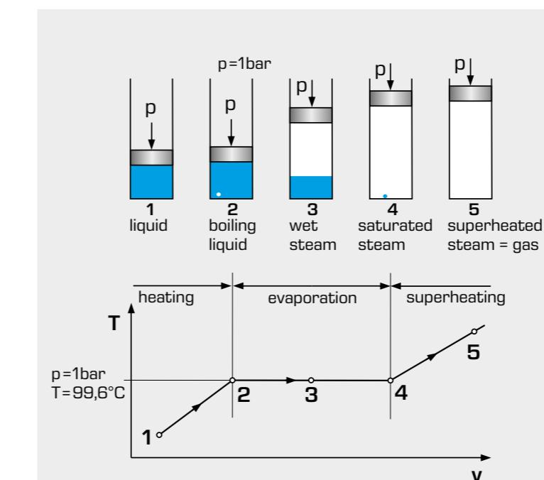
Evaporation of water: change of state when heating water under constant pressure  $p = 1\text{ bar}$
