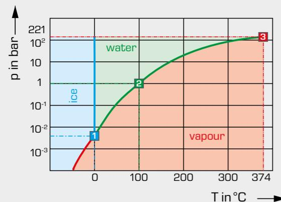
Temperature-pressure diagram of water
