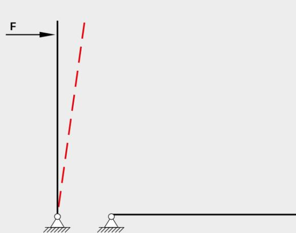
Bar does not return to the starting position after the load is removed and does not stay in the position it assumed while the load is being applied. The bar falls over.
