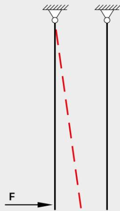
Bar returns to its starting position after the load is removed.
