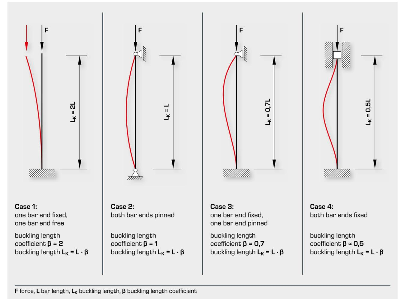
Determining the buckling force  $F_K$
