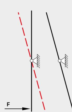
Bar remains in the new position after the load is removed.
