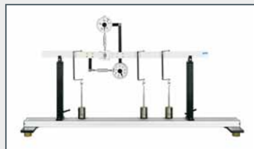
WP 960 Beam on two supports: shear force & bending moment diagrams
