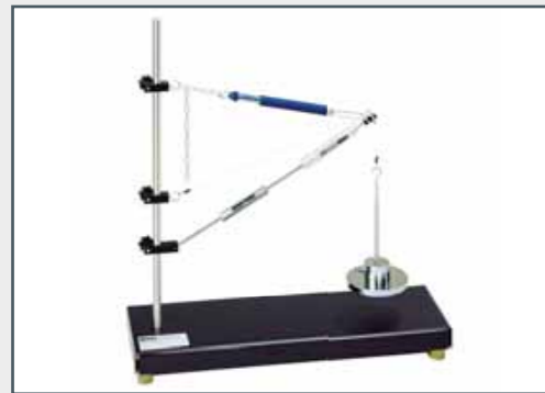
TM 115 Forces in a crane jib
