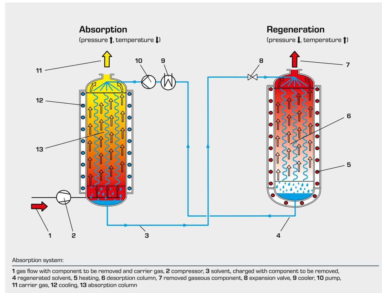
An appropriate solvent is used, depending on the gaseous component to be removed. The solvent selectively dissolves the gaseous component i.e. the solvent primarily absorbs the component(s) to be removed and not the carrier gas. High pressures and low temperatures enhance absorption. Depending
