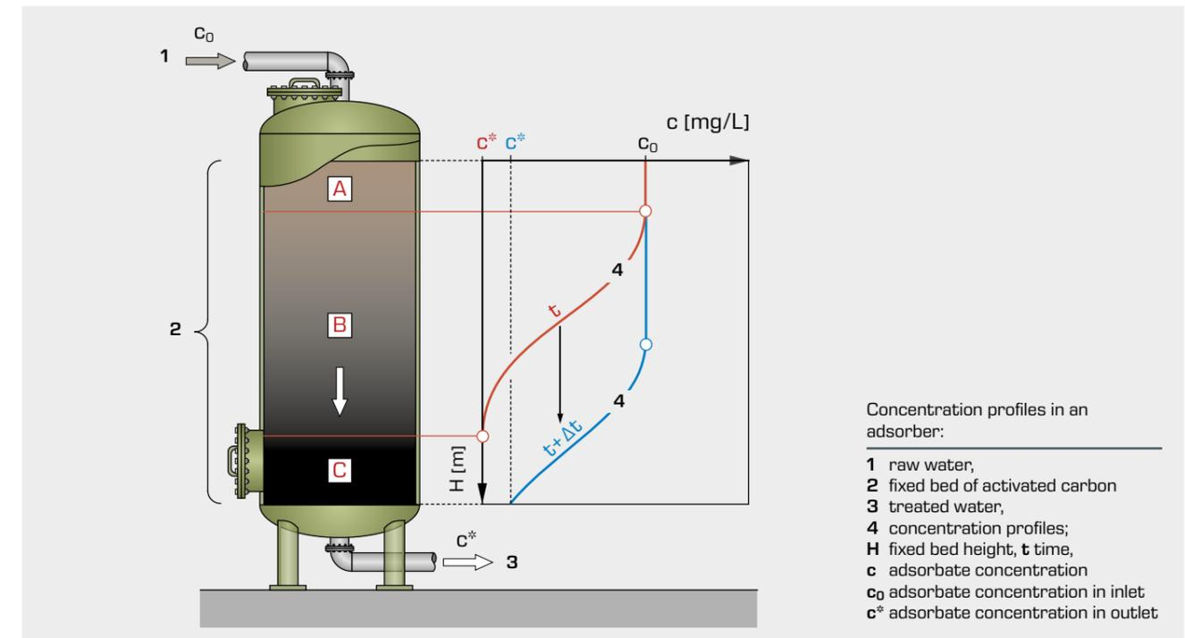
Adsorption is mainly implemented with continuous-flow adsorbenters. In this case, the concentration profile marked in red on the illustration is established after the time t. It corresponds to the trend of the adsorbate concentration in the water along the fixed bed.
