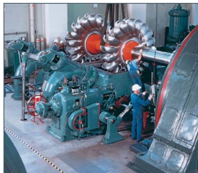
Assembly of a Pelton turbine at the Walchensee power plant in Germany (Voith Siemens Hydro Power)
