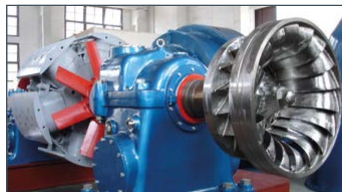
Francis turbine, deinstalled
