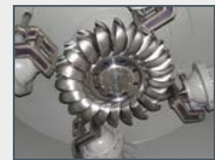
The water jet changes direction in the blade without changing velocity
