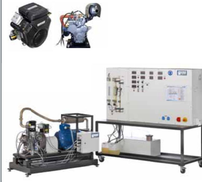
CT 300 Engine test stand, 11 kW
