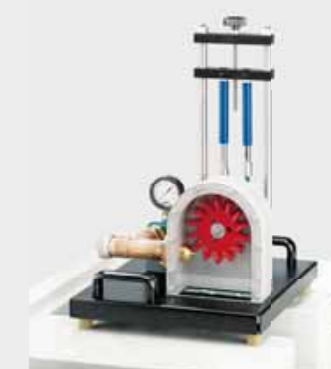
HM 150.19 Operating principle of a Pelton turbine
