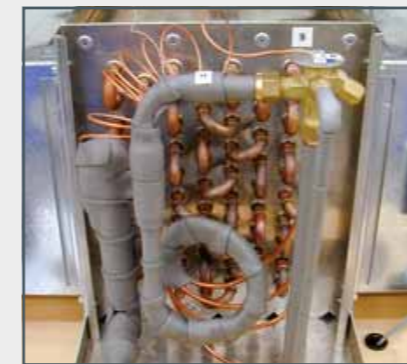
Direct evaporator as air cooler
