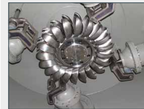
Rotor with double buckets as blades and needle nozzles
